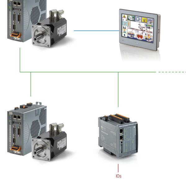
SBD/PLC SmartDrive: the brushless drive is used as a controller in CANopen for the management of I/O peripherals such as RP064 I/O and/or other SBDs.
