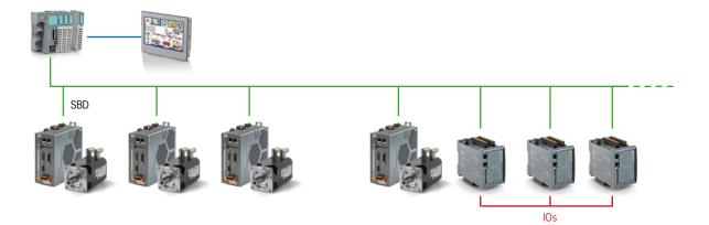
In the classic configuration SBD is suitable for the automation of complex multi-axis machines in combination with FCT640 controller, programmable in CODESYS, and I/O peripherals such as RP064 I/O.
